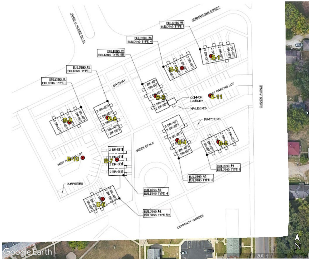
Figure 4: 2022 Google Aerial – Boring Locations
